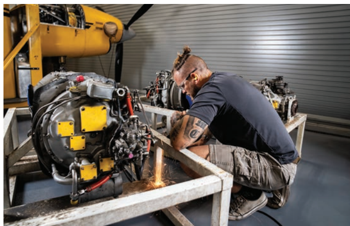
Lorenzo Walker students modify and raise the base housing the two turbine engines funded by the Collier Community Foundation to allow mobility for easy accessibility in learning rotorcraft fundamentals.
